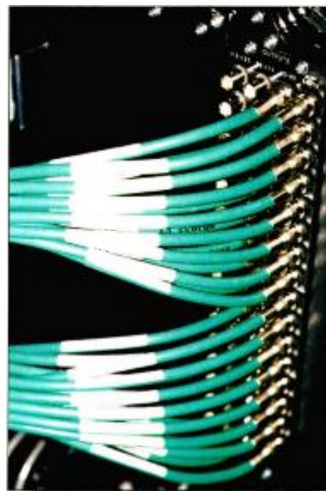
Make sure that your BNC connectors are up to the task of routing your signal. Many low-end BNC connectors are not capable beyond 1GHz. Photo courtesy of Commscope.
