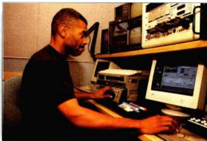
The utility of the NewsEdit system is largely due to the similarity of its tools to those used in tape-based editing, allowing those without nonlinear editing skills to transition easily to its use.
