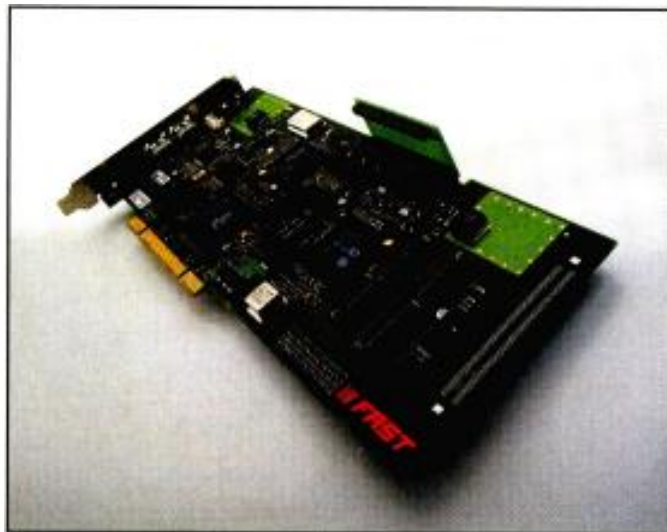
Fast Multimedia's silverDV. The DV option allows silver. users to input DV footage directly from DV cameras.
